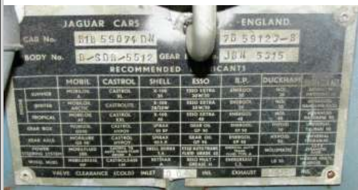
The chassis plate of South African built B1B59074DN. Note the chassis number is in the proper location and the Jaguar Body Number has 'SDB' added between the 'B' prefix and the number.
