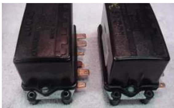
Left: Original RB.340 Control Box with cover held on by screws. Right: Replacement unit with riveted cover.
